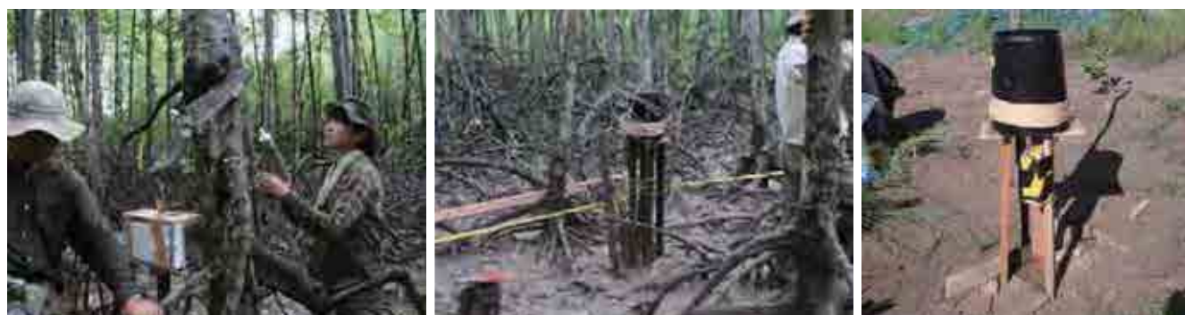
Figure 29 Set up of stemflow trap (left), throughfall trap (middle) and gross precipitation trap (right) at the MEET Center (Saitoh, 2008)
