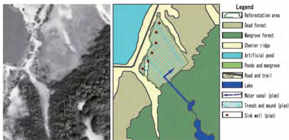
Figure 3.5 An aerial photograph (left) and proposed mangrove rehabilitation scheme (right) of Block C in Celestun
