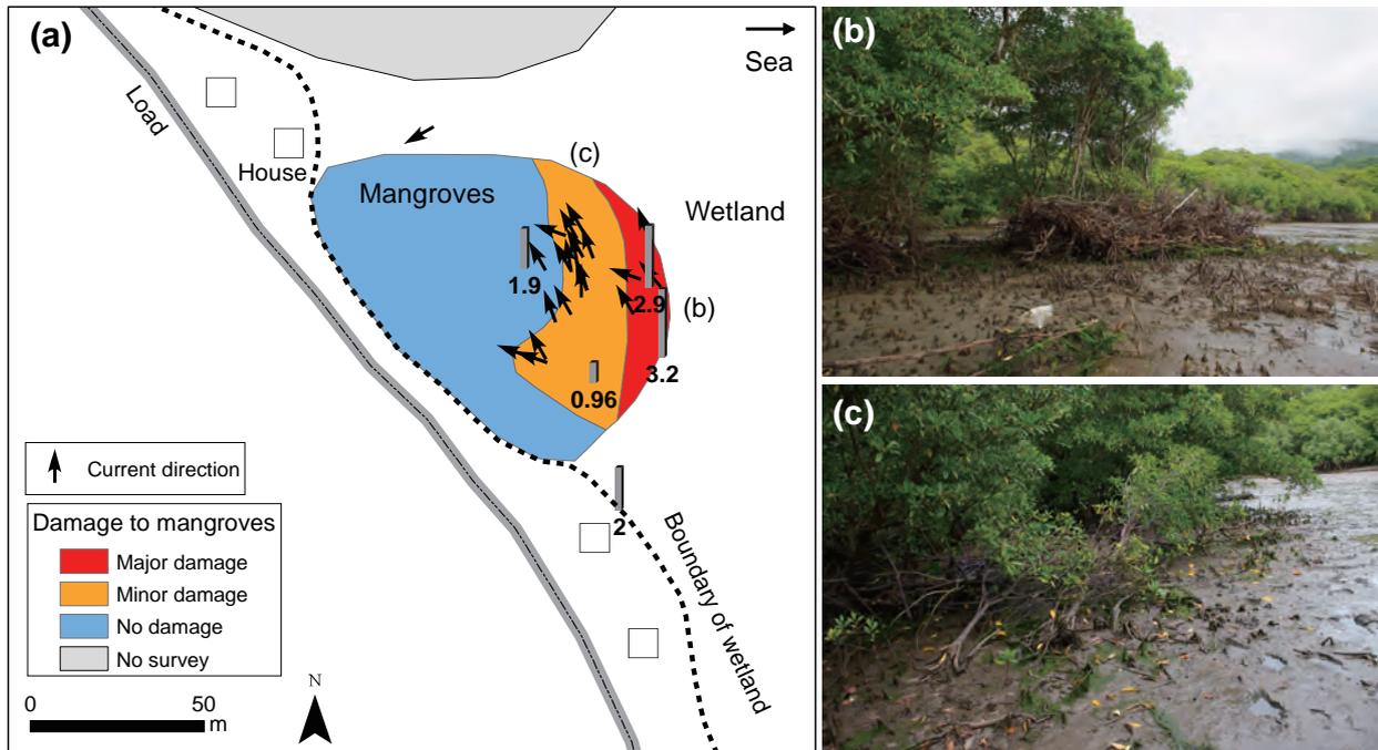
**Fig. 3** Tsunami damage on mangrove forest in Matafaa. (a) Tsunami height (m), current direction (the arrows do not include a flow strength) and mangrove damage. (b) and (c) show damage to mangrove trees at (b) and (c) in map (a).
